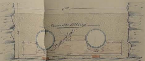
Section showing method of supporting pipes and concrete filling in new channel
