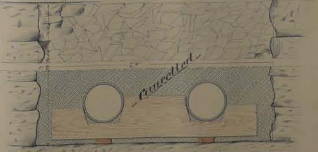
Section showing method of supporting pipes and clay in stone filling in the channel
