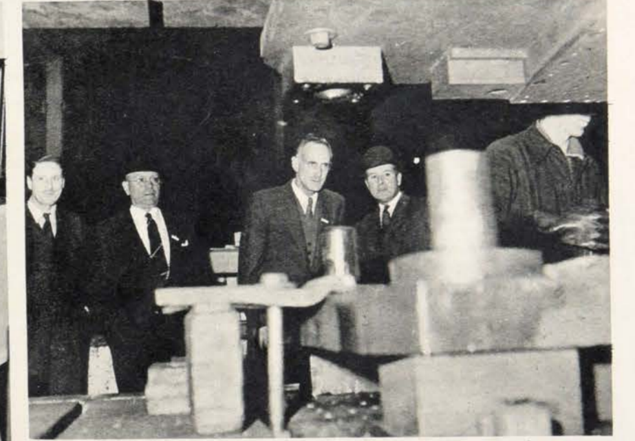
A GIANT PRESS: In the foreground are the dies of a 3,000-ton clearing press, as members of the Canadian Trade Mission watch the pressing of heavy parts for railway wagons being made at the Wolverhampton works of John Thompson Ltd.
