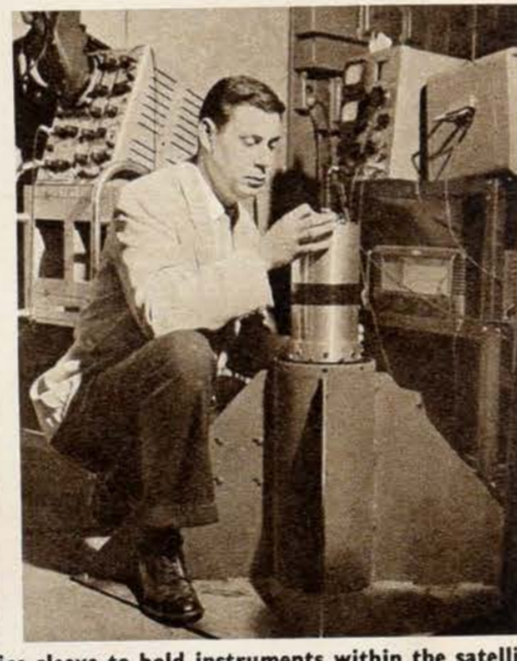
PRECISION WORKERS: On extreme left—A fibreglass lattice sleeve to hold instruments within the satellite is carefully machined in the Jet Propulsion Laboratory. Centre—The sleeve is inspected by a technician. On right—The finished sleeve with its delicate instruments within is prepared for a "shake test."
