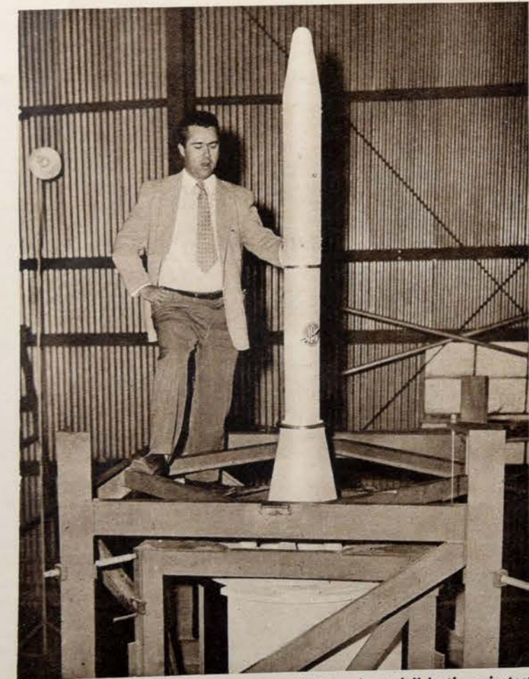
THE FINAL ASSEMBLY: Positioned on a "balancing tub" in the spin test rig, the satellite is inspected by a technician of the Jet Propulsion Laboratory. The satellite is stabilised by its spin like a rifle bullet.
