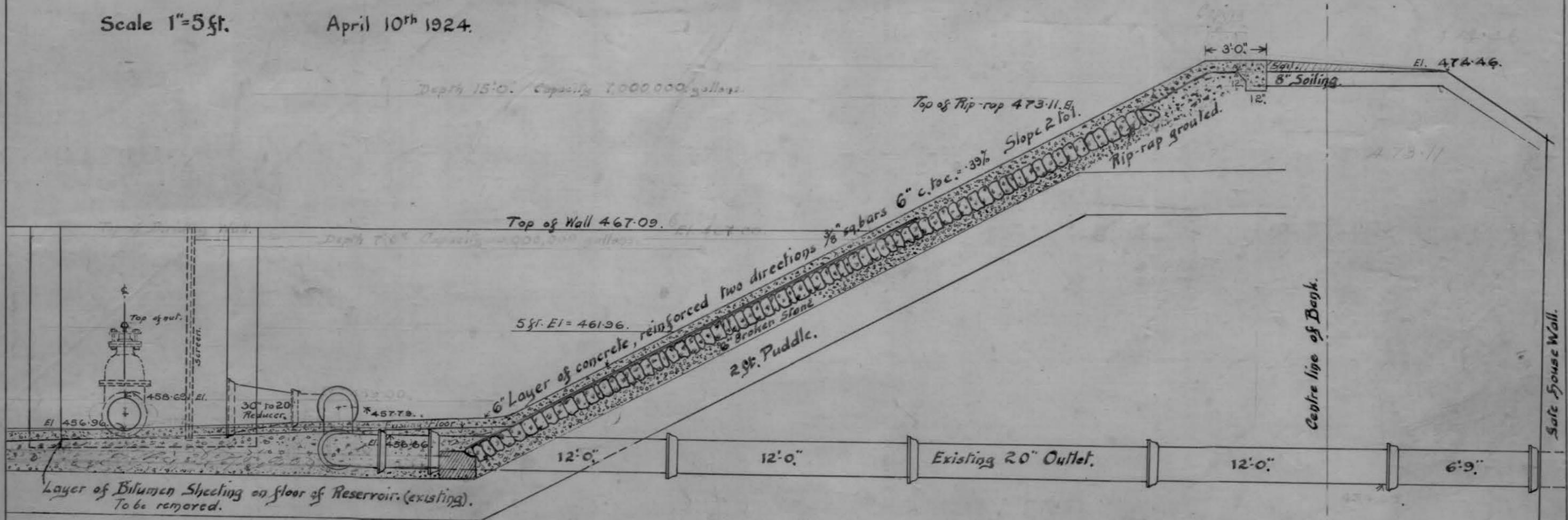
Portland cement concrete on floor and sides of reservoir to be 1:2:4 mix.
